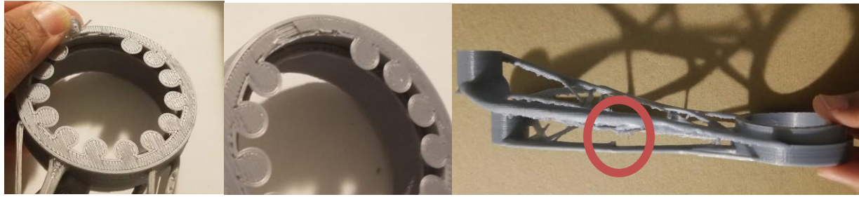
Figure 30: Removing support material causing damage
